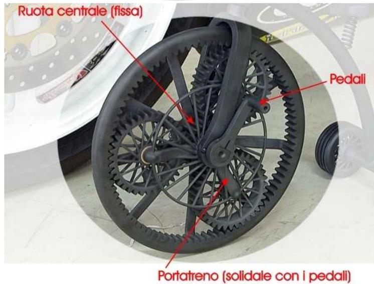
**Fig.2** – Particular of the system of transmission of the motion.
