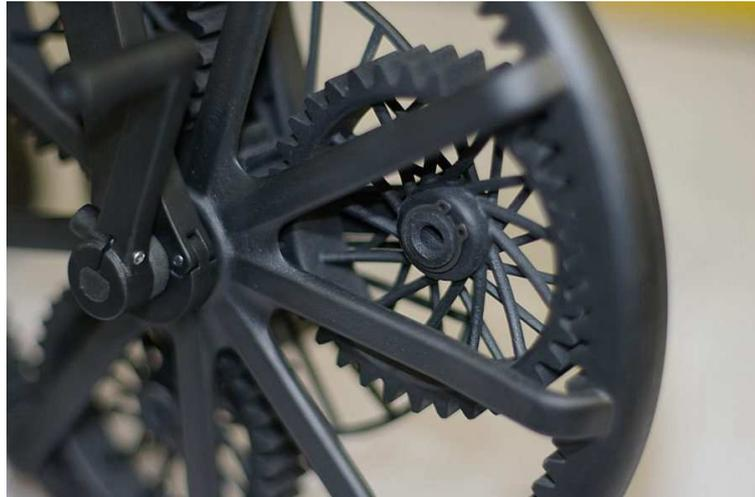
**Fig. 5a/b/c** – Front wheel assembling system. To be noticed the blocking system of the wheels on the axles through snap ring.
